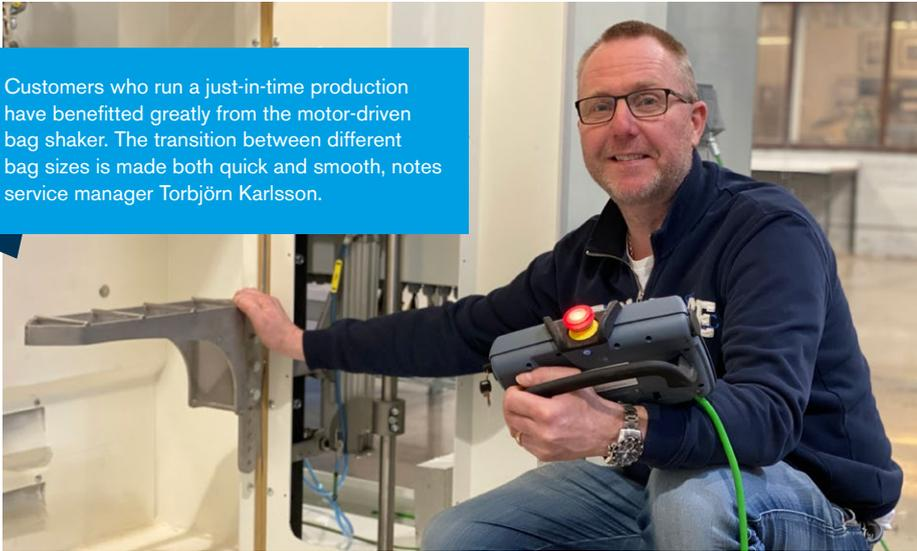
**Shaking the bag after it has been filled compresses the contents and creates a higher fill density. This is important for many of Vebe's customers.**
