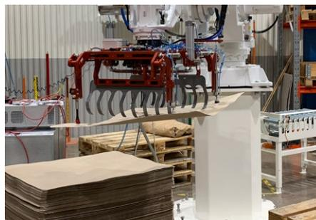
One of the finesses of the new robotic handling of slip sheets is that the sheets no longer require manual lifting. This simplifies the process. It also removes a production step which creates a more ergonomic setup. ■
